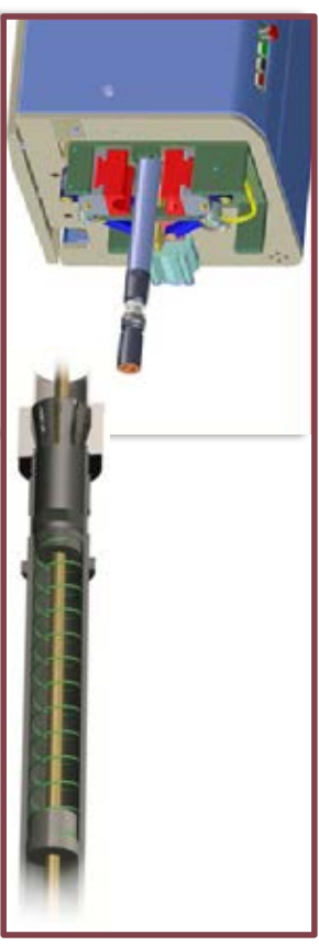
Oil bath lubricated pneumatic bar centering device between loader and lathe and automatic spring bushing inside the lathe spindle
